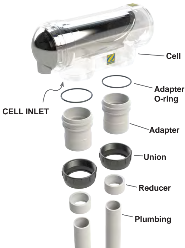
Figure 5. Cell Plumbing Assembly
