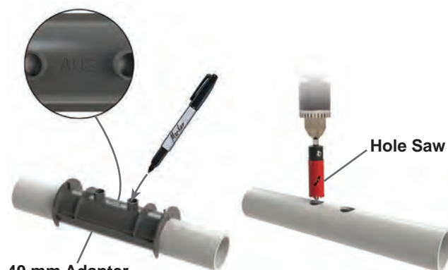
40 mm Adapter Figure 13. Mark and Drill Pipe
