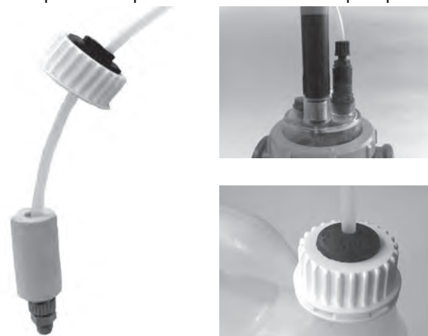
Figure 22. pH- Intake Connections
